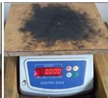
Fig 9. Balance scale for water and fuel measurement
