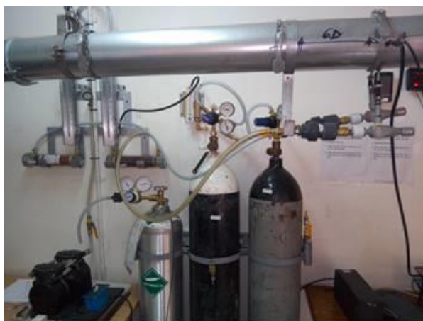
Fig 6. PM Sampling train and Calibration gases
