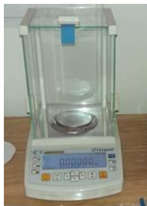
Fig 8. Microbalance scale for filters
