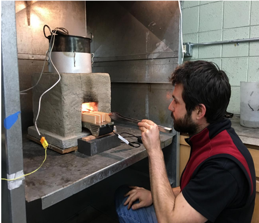
Figure 1 The ZHSC Jet-Flame in the Clay/Sand 15 Brick CQC Rocket stove with pot skirt.
